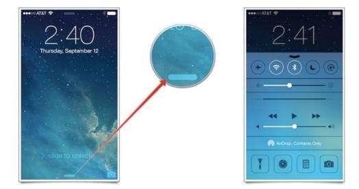
Place your finger below the screen (on the bezel as indicated). When the grabber appears, place your finger on it and slide your finger up onto the screen to reveal Control Centre. If you have a cover on your device it may interfere with this action.
